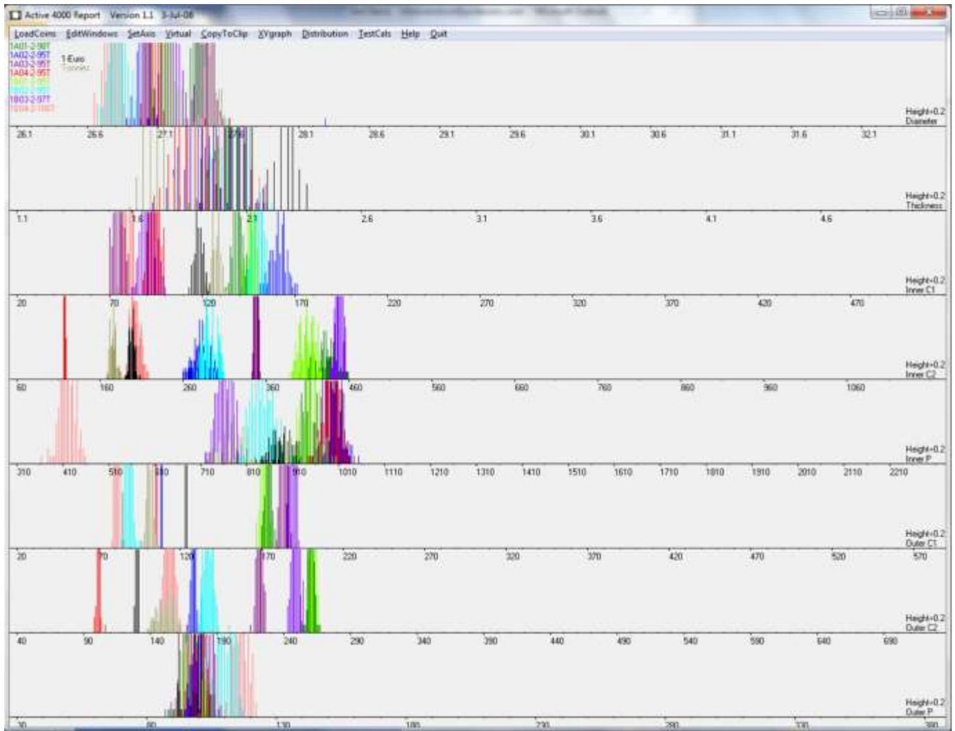
It is interesting to note that all the 7 different combinations of bimetal coins resulted in their own distinct signature in the OC2 plot. Combinations 1A01 and 1B01 in which zinc was utilized in both core and ring overlapped in the EMS signature. As the plated finish on 1A01 and 1B01 were essentially reversed, the result implies that plated finish had little role, if any, in driving the EMS signature on these coins.
