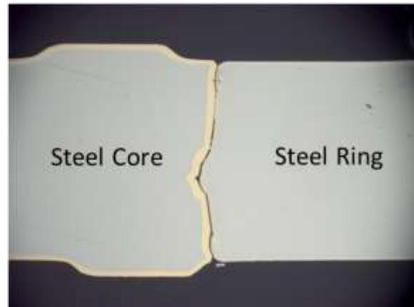
While the material from the ring seems to fill the groove in the core well, there does not appear to be a significant difference in the groove filling or the groove shape compared to other samples (1B02 and 1B03) that may explain the observed higher separation force in these coins.
