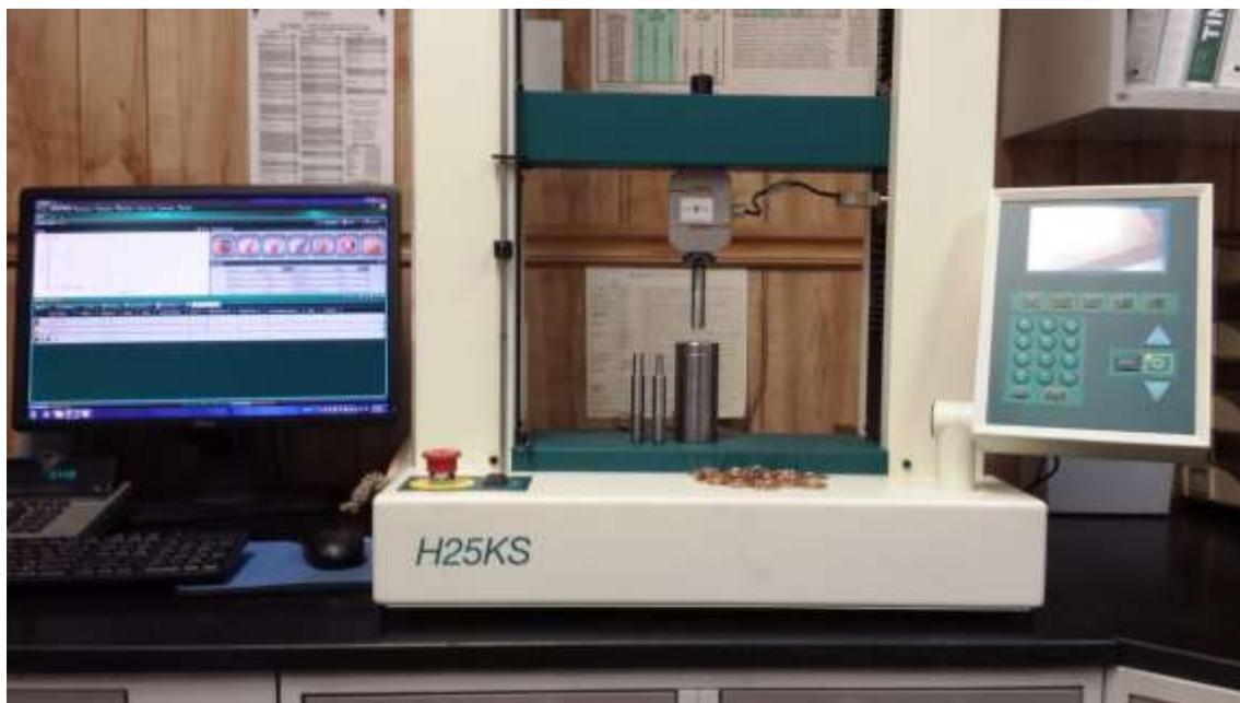
Several factors play a role in the accuracy of test results and the effect of these factors was examined, the factors included; piston travel speed, the ratio of piston diameter ( $D_p$ ) to diameter of core ( $D_c$ ) and the clearance between coin ID and fixture ID ( $CL = D_f - D_{\text{coin}}$ )
