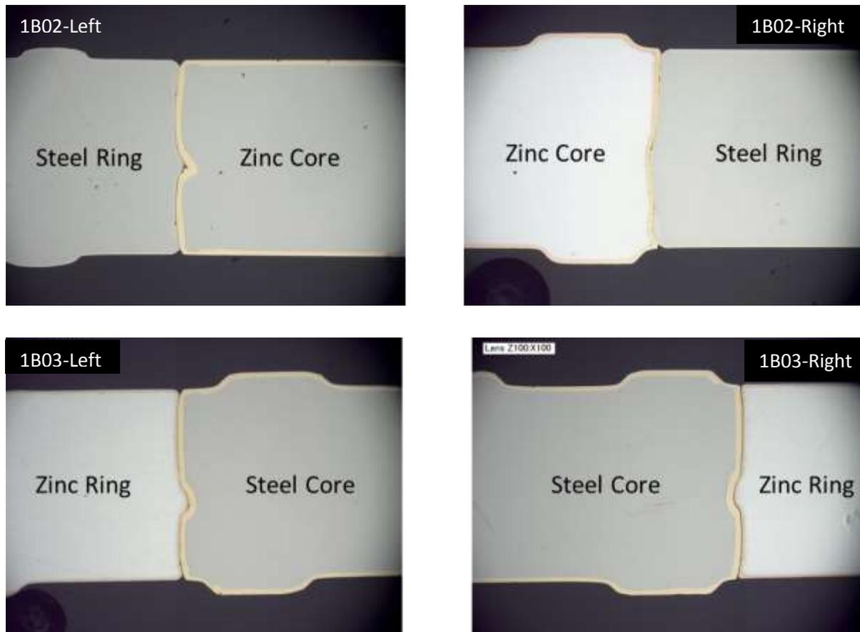
From the above figure it can be seen that the groove in the core has been filled well with the zinc material in both 1B02 and 1B03 sets. Given that the materials set for ring and core combination is same for these sets, it is not surprising to see the separation force numbers are also similar.
