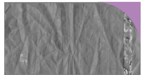
3D processed image of printed banknote. With such an image, captured by Snowfish, the three dimensional aspects of a note can be easily quantified.
