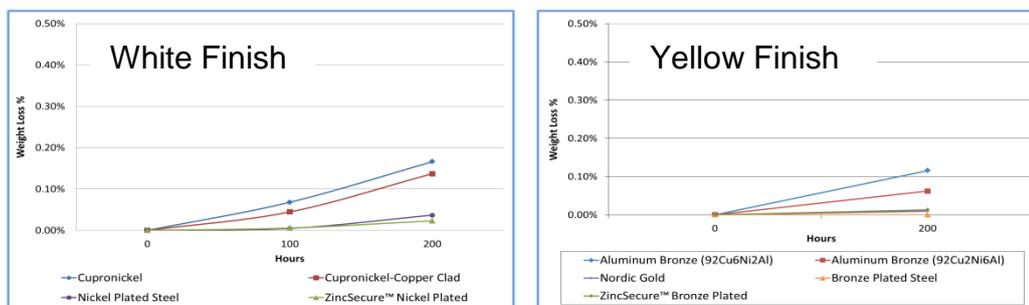
Similar to the wear test in Figure 2, the wear results in this dry tumble test (Figure 3) demonstrate that for all nickel plated product, whether zinc-based or steel-based, the wear rates are comparable and exceptionally lower than the through alloy cupronickel or cupronickel-copper clad material.
