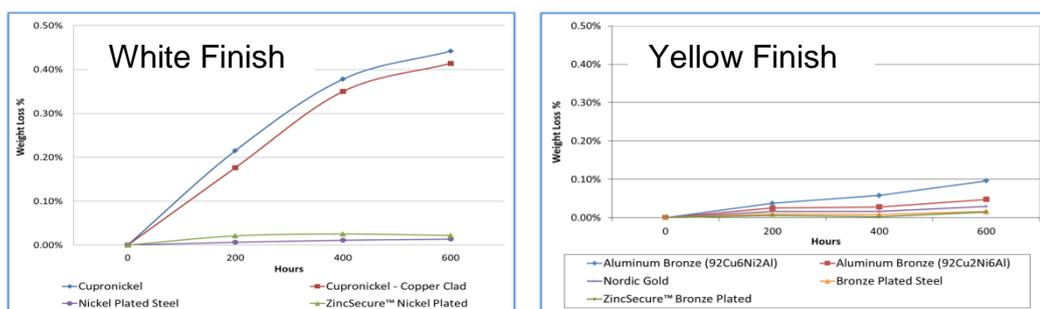
The resulting wear results for the white finish samples are illustrated in Figure 2. As can be seen, the wear results for all nickel plated product, whether zinc-based or steel-based are comparable and exceptionally lower than the through alloy cupronickel material.
